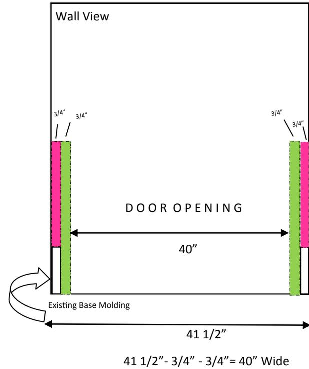
My base molding is 3/4". First piece makes base and wall even, the second door jam hinge piece will make opening measurement for door -3/4" off the total. For example my measurement for piece 4 and 5 for the door will be 3/4" + 3/4" = 1 1/2" off the total.
